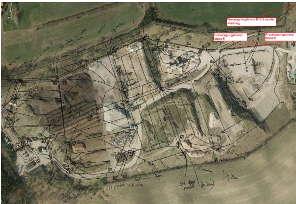
Figure 3.3: Overview of the leachate collection system at Skaarup Landfill, including the sampling points for leachate from Cell 5, Cell 6 and the combined leachate from Cells 1 to 4, 5 and 6.
