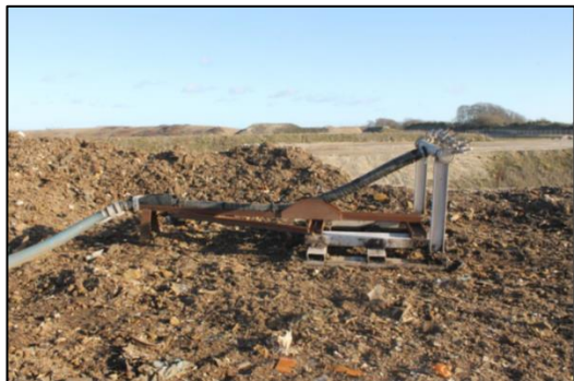
Figure A6.2: The leachate spreading units at Reno Djurs (from Rolsted and Rosendal, 2016).
