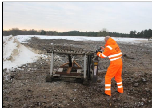
Figure A6.2: The leachate spreading units at Reno Djurs (from Rolsted and Rosendal, 2016).
